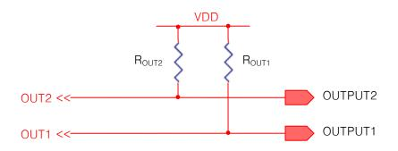
The OUT1 and OUT2 have open drain output structure. For this reason, the connection of pullup resistor R<sub>OUT</sub> is required between OUT1, OUT2 and VDD. The maximum output sink current is 4mA, so over a few k  $\Omega$  must be used as  $R_{OUT1}$  and  $R_{out2}.$  Normally 10k  $\Omega$  is used as  $R_{OUT1}$  and R<sub>out2</sub>. The reset value of OUT1 and OUT2 is high in normal situation, and the value is low when a touch is detected on CS1 or CS2.
