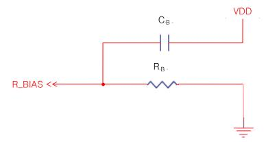
The R\_BIAS is connected to the resistor to decide the oscillator and internal bias current. The sensing frequency, internal clock frequency and current consumption are therefore able to be adjusted with R.B.. A voltage ripple on R\_BIAS can make critical internal error, so C.B. is connected to the VDD (not GND) is recommended. (The typical value of C.B. is 820pF and the maximum Value is 1nF.)
