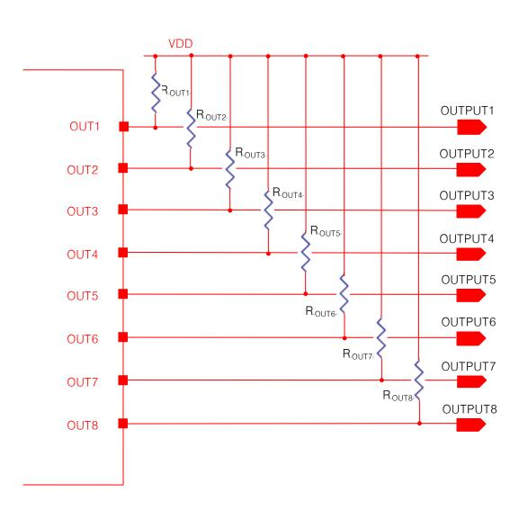
The OUTPUT pins have an open drain structure. For this reason, the connection of pull-up resistor R<sub>-OUT</sub> is required between OUTPUT and VDD. The maximum output sink current is 4mA, so over a few k $\Omega$  must be used as R<sub>OUT</sub>. Normally 10k $\Omega$  is used as R<sub>OUT</sub>.
