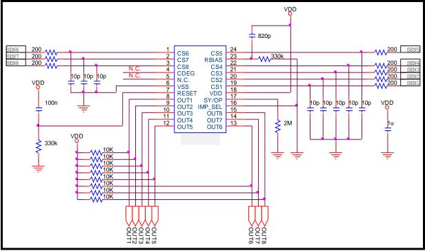
TS08NE(24SOP) Application Example Circuit
