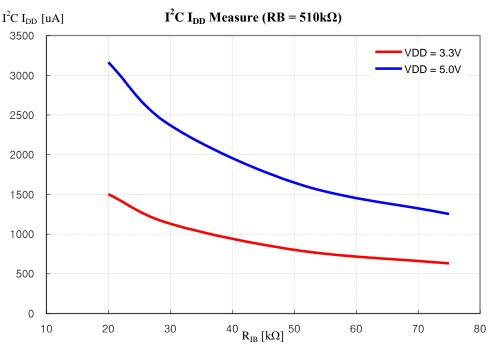
I2C Block operation current consumption curve
