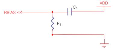
The RBIAS is connecting to the resistor to decide the oscillator and internal bias current. The sensing frequency, internal clock frequency and current consumption are therefore able to be adjusted with R<sub>B</sub>. A voltage ripple on RBIAS can make critical internal error, so C<sub>B</sub> is connected to the VDD (not GND) is recommended. (The typical value of C<sub>B</sub> is 820pF and the maximum Value is 1nF.)
